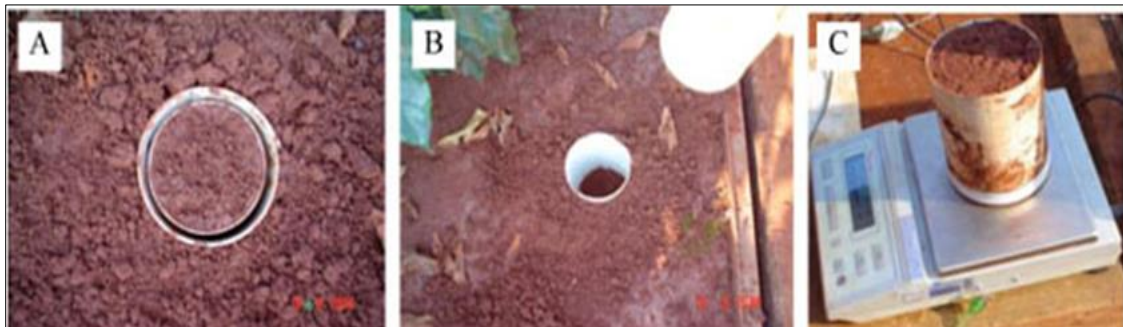
Figure 3 Micro-lysimeter installed with the outer envelope in detail (B) and micro-lysimeter weighing (C). (Source: Danilton et. al [7])
