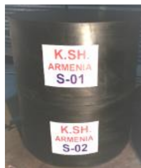
Figure 12 Views of the tested and labeled SILRSBs; these isolators will be located by upper and lower recesses provided by annular steel rings bolted to outer steel plates which are connected to the reinforcement in the upper and lower continuous beams; the isolators themselves are not bolted to the structure
