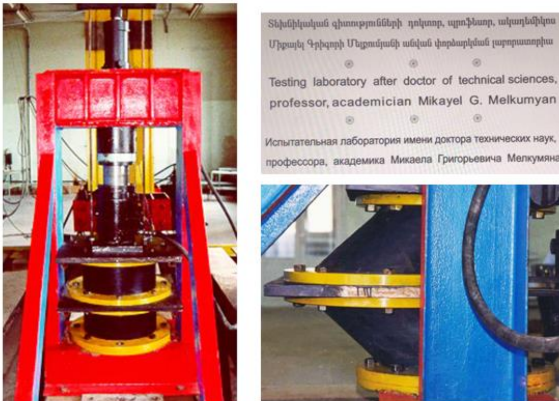
Figure 11 Facilities in the laboratory named after the author of this paper and designed by him for testing of different types of the seismic isolation laminated rubber-steel bearings
