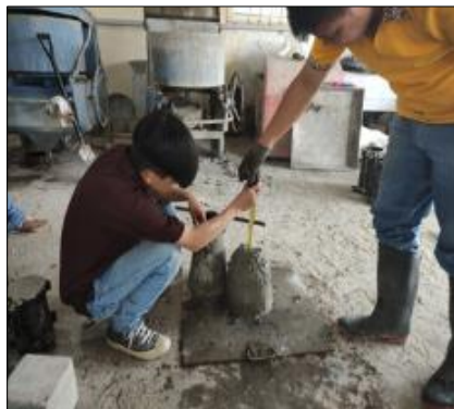
Figure 2 Slum Measurement And Making Concrete Samples
