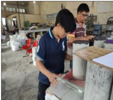
Figure 3 Compressive Strength Measurement And Testing Process
