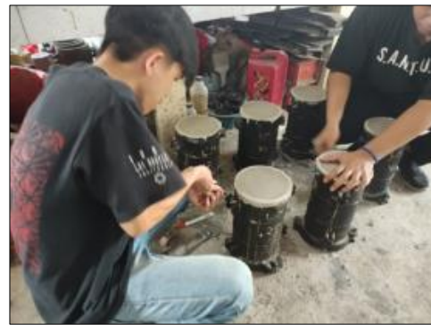
Figure 2 Slum Measurement And Making Concrete Samples
