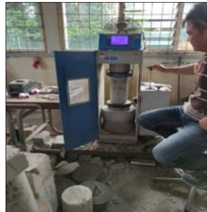
Figure 3 Compressive Strength Measurement And Testing Process
