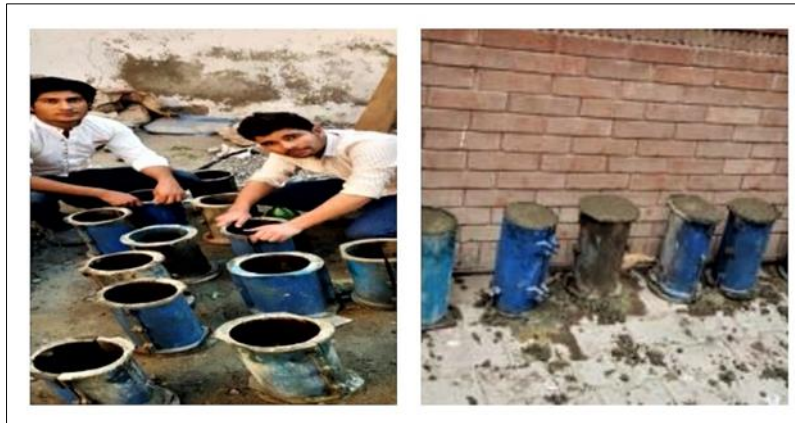
Figure 1 Casting of cylinders
