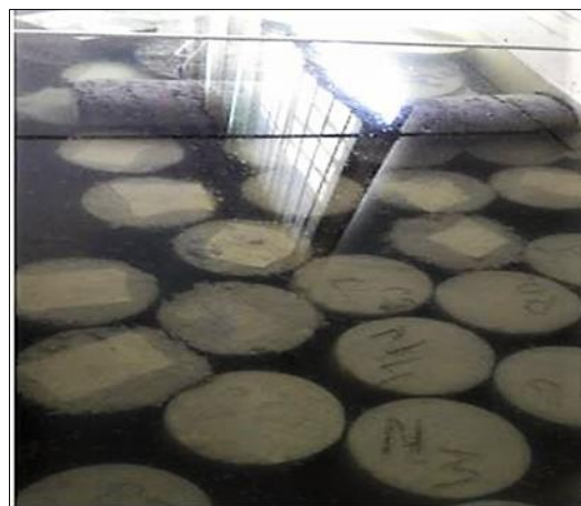
Figure 2 Curing of cylinders
