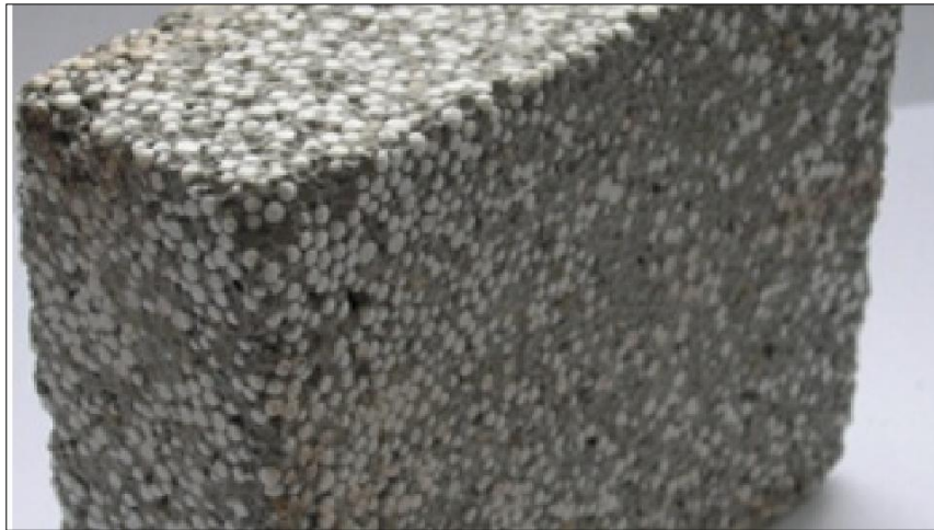
Figure 6 Recycled Expanded Polystyrene Light Weight Block (Source: [65])
