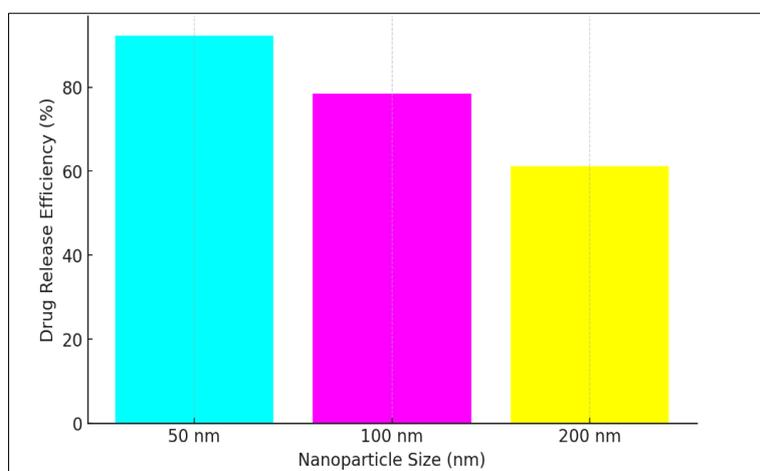
**Figure 6** Relationship Between Nanoparticle Size and Drug Release Efficiency. Smaller nanoparticles facilitate faster drug release compared to larger counterparts
