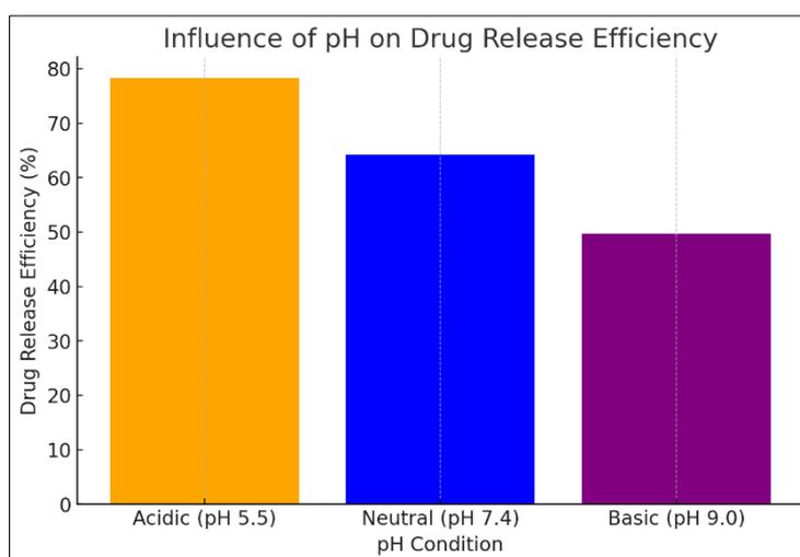
**Figure 5** Influence of pH on Drug Release Efficiency. Acidic environments enhance drug release, likely due to polymer degradation and solubility effects
