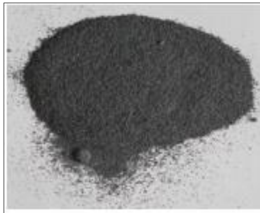
Figure 2 Fly ash particles (Size -45 to80 microns)
