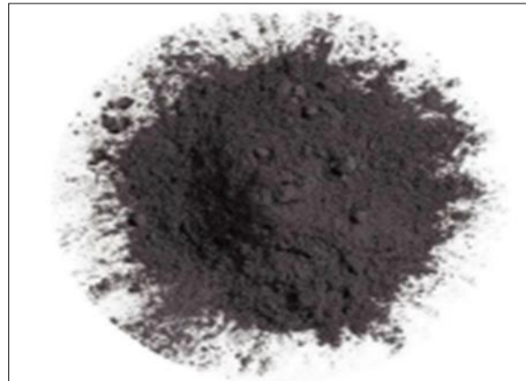
Figure 3 Fly ash particles (Size -25 to 45 microns)
