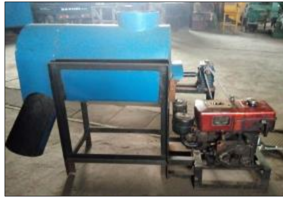
Figure 1 Pictorial View of the NCAM coconut dehusking machine
