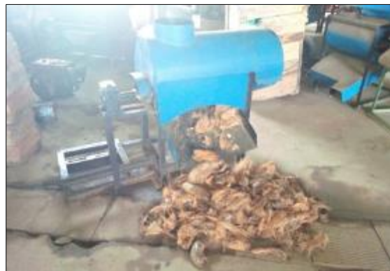
Figure 3 Coconut dehusking machine during the performance test
