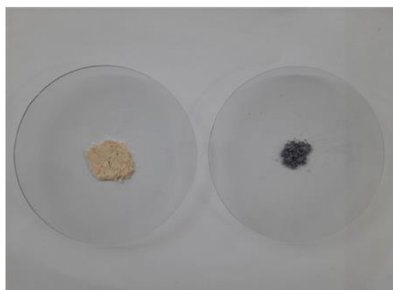
Figure 3 The CBP before (a) and after (b) being used for the adsorption of sulphur blue dye
