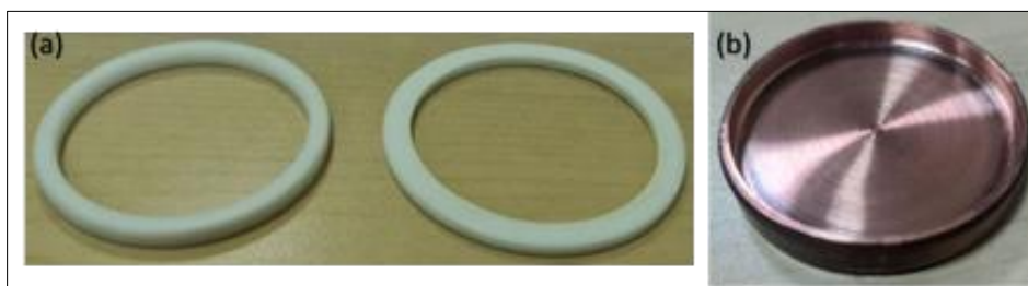
Figure 1 (a) PTFE deformable die rings, used for the pressing of the targets. On the left-hand side, the ring before pressing, and the right-hand side corresponds to the ring after pressing the powder. (b) Copper holder used as a protective and provider of enhanced contact between target and sputtering gun
