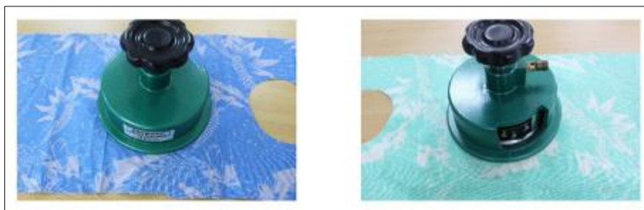
Figure 2 Printed fabric sample cutting with GSM cutter
