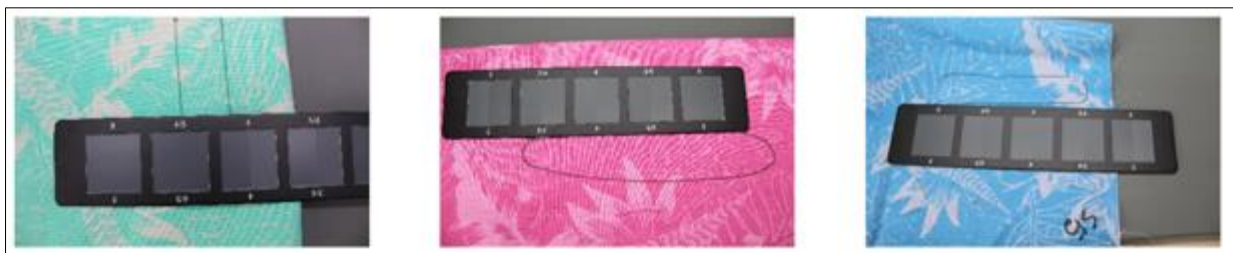
Figure 5 Color change evaluation of rubbing fastness test of printed fabric sample
