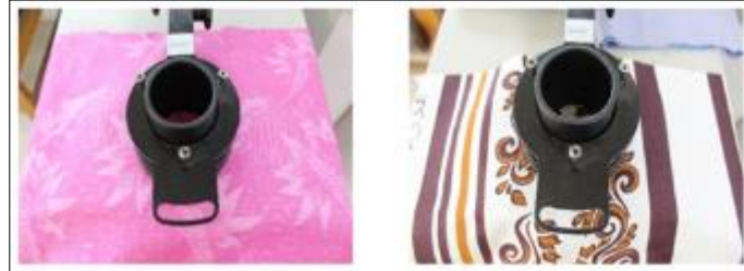
Figure 7 Air Permeability test of printed fabric samples
