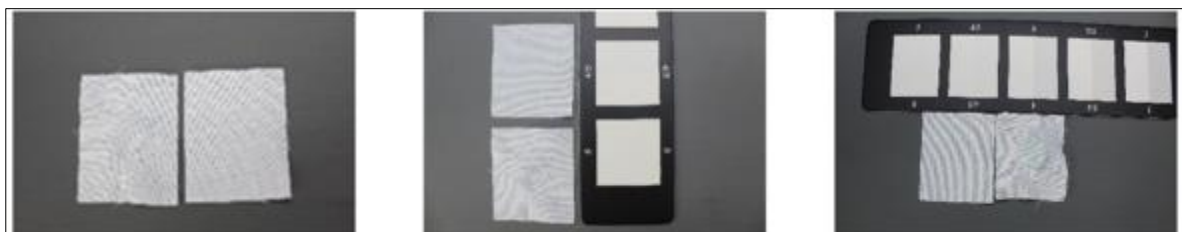
Figure 6 Staining evaluation of rubbing fastness test of printed fabric sample
