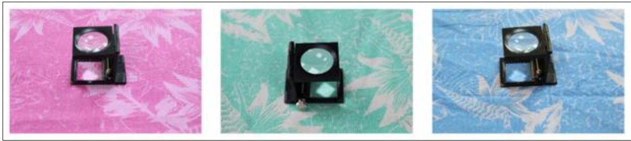
Figure 1 EPI and PPI measurement with counting glass
