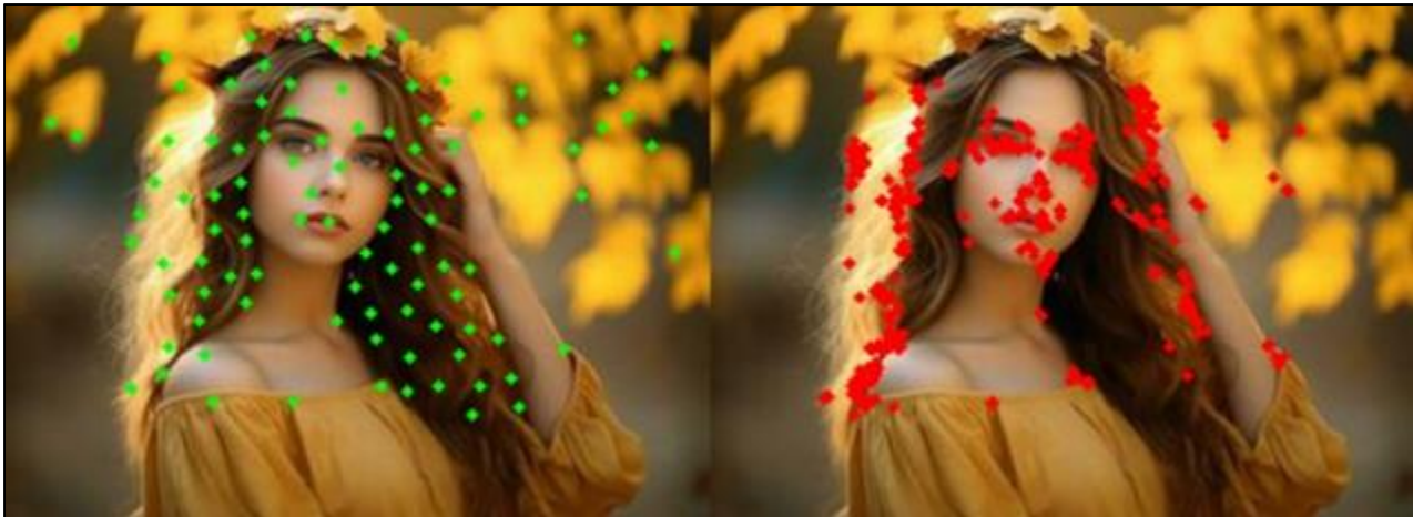
Figure 6 Multi-Channel and Multi-Featured Extended ORB with Gabor Filter and Non Maximum Suppression keypoints vs Simple ORB keypoints
