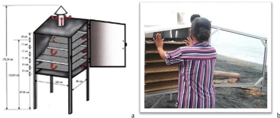
Figure 2 Drying chamber design based on ergonomics principles through worker anthropometric data [7]
