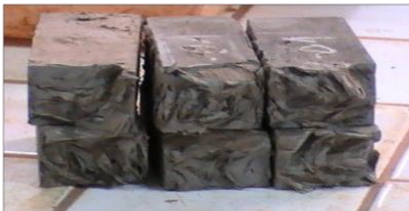
Picture 4 Height (8) years old wood concrete test tubes after flexion tests
