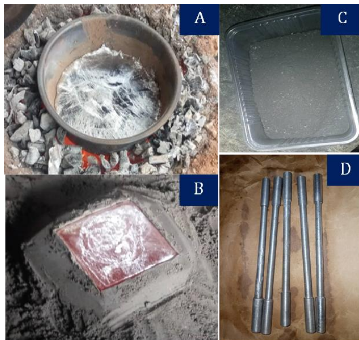
Figure 2 Process of producing the ingot. (A) melting of the discarded pistons (B) produced ingot (c) grinded carbon rods of the batteries (D) Machined specimen for experiment.
