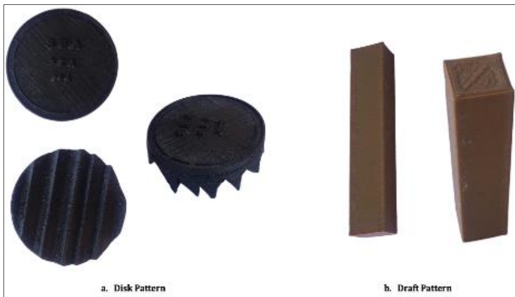
Figure 2 3D-Printed Patterns. (a) Disk Pattern. (b) Draft Pattern
