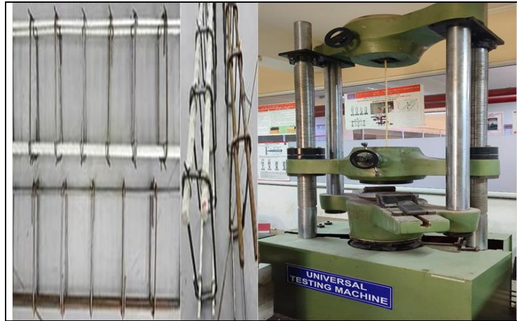
Figure 22 Tensile test of GRPF bars
