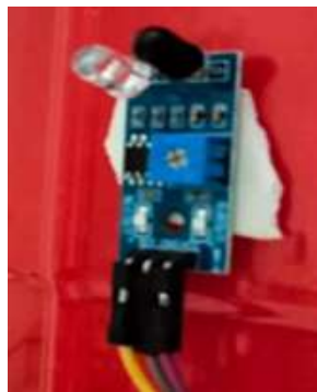
Figure 2 IR Proximity Sensor
