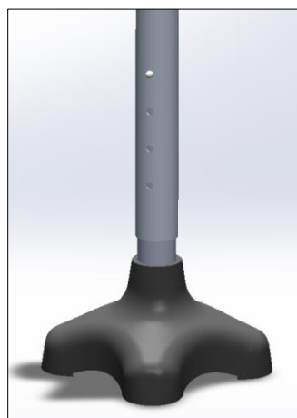
Figure 8 Close up of cane base assembly and second-third tube joint
