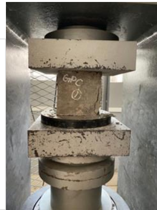
Figure 1 Compressive Strength of the Specimens for 28 days
