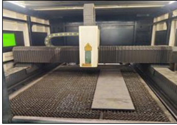
Figure 3 CNC laser Cutting machine
