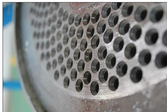
Figure 5 Normal inlet countersink of pressing channels
