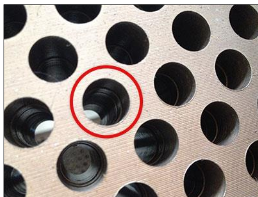
Figure 6 Detail of the outlet relief of the pelleting die
