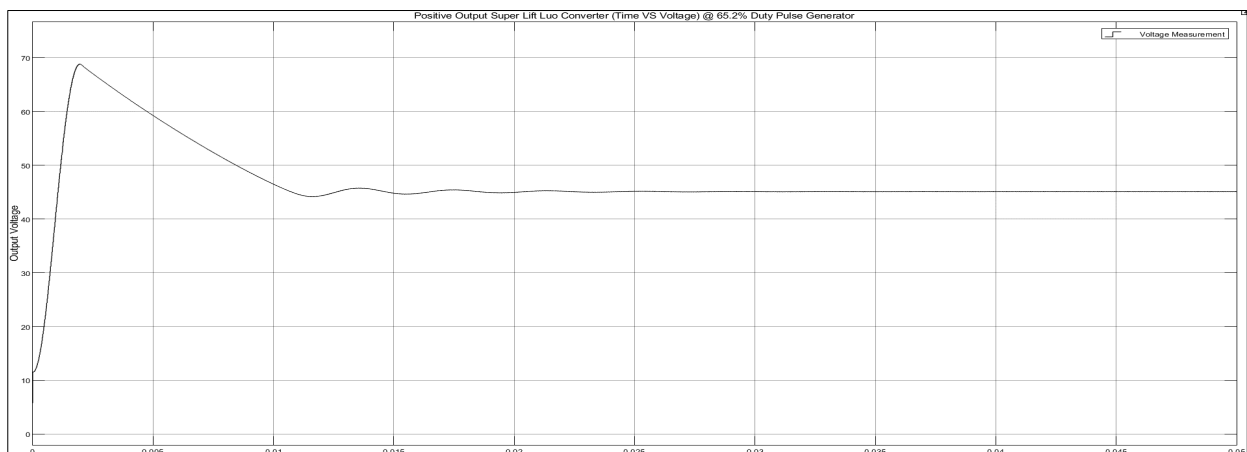
Figure 7 Positive Output Super Lift Luo Converter Time VS Voltage at 65.2% Duty Pulse Generator
