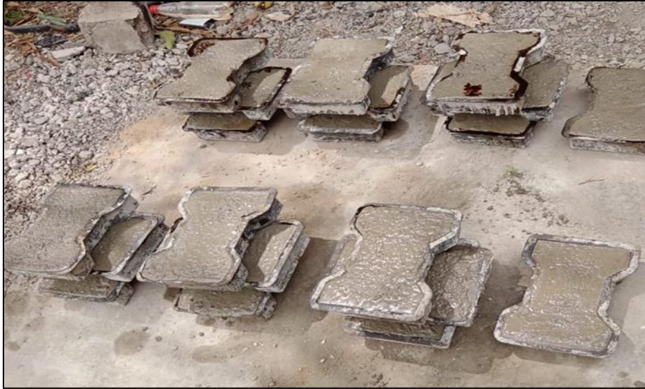
Figure 2 Interlocking paving stones
