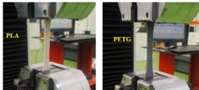
Figure 5 Tensile setup used for testing.
