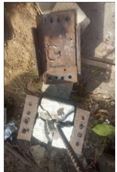
Figure 6d Inserted rebars in the concrete cubes
