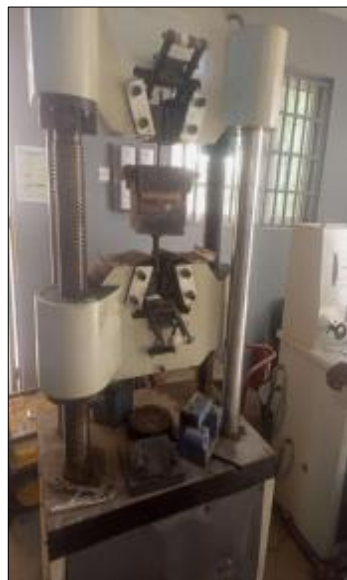
Figure 6c The pullout set-up on the universal testing machine
