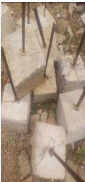
Figure 6a Inserted rebars in the concrete cubes
