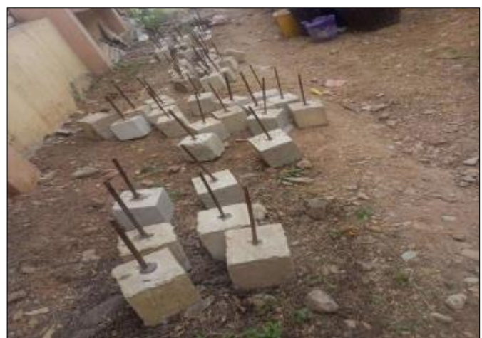
Figure 5 Application of Hilti RE100 Adhesive for Embedding Rebars into the Concrete Cubes
