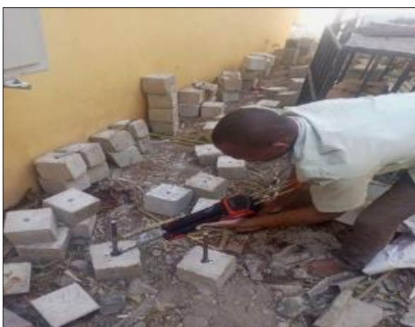
Figure 5 Application of Hilti RE100 Adhesive for Embedding Rebars into the Concrete Cubes
