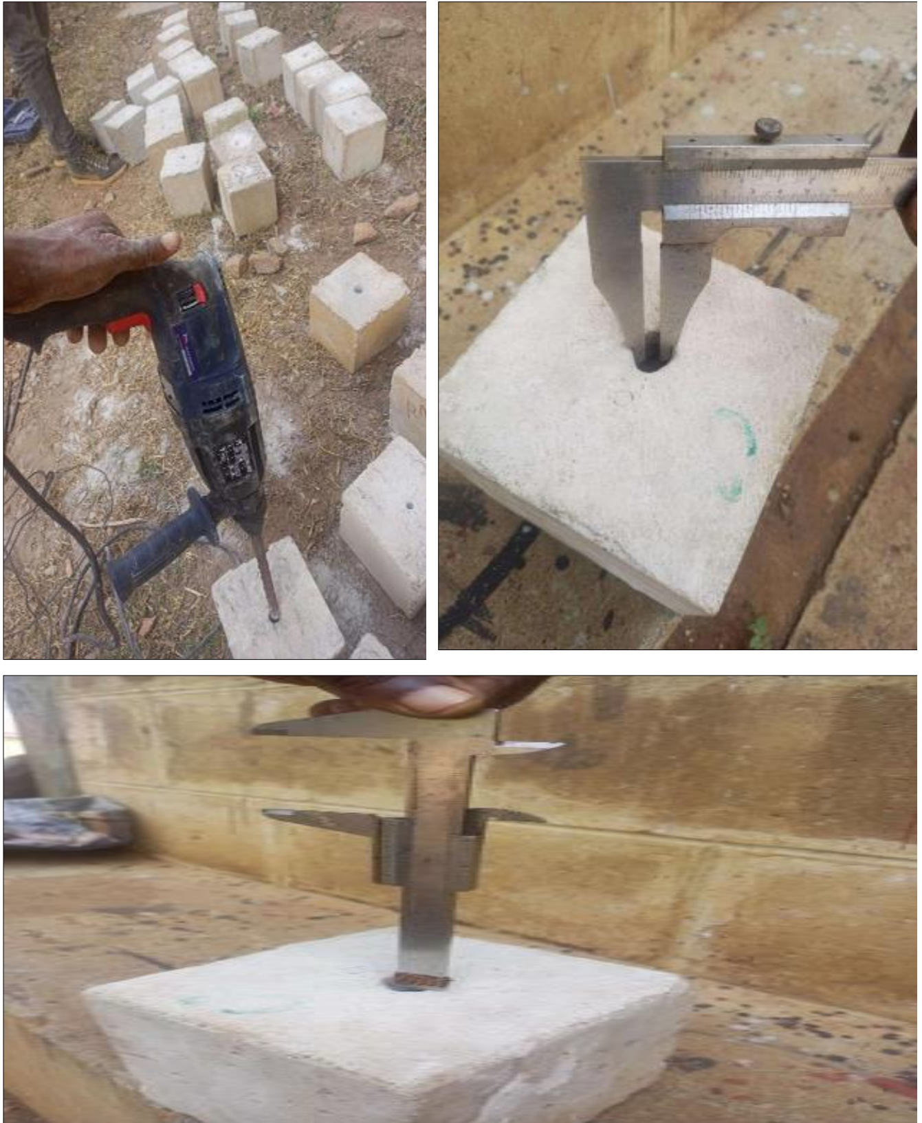
Figure 2 Marking of the Centre of Cubes Samples and Drilling of Embedment Length, Measuring of Internal and External Diameter respectively
