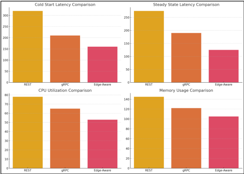
Figure 2 Memory Usage Comparison: Memory consumption across REST, gRPC, and Edge-Aware architectures. REST incurs higher overhead, gRPC is more efficient, and Edge-Aware further reduces usage by offloading tasks to edge servers
