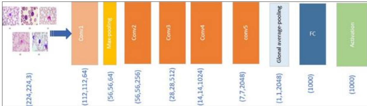
Figure 3 Model architecture of ResNet50
