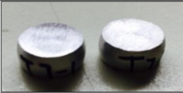
Figure 33 Reduction in height of AA7055-T7751 Aluminium alloy
