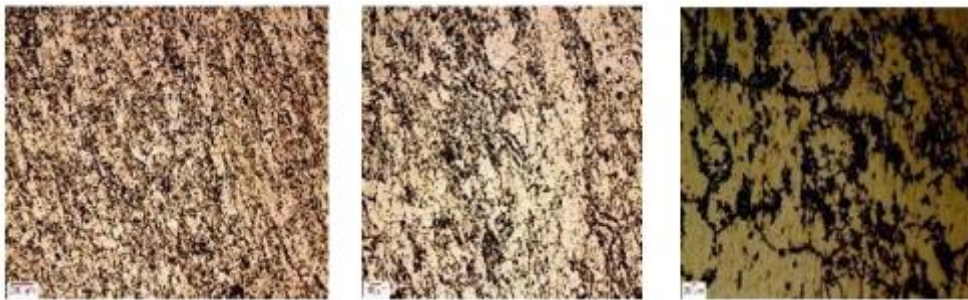
Figure 46 Microstructure of AA7055-T6 alloy at impact pressure of 160kPa (C4) at magnifications of X50, X100, X500
