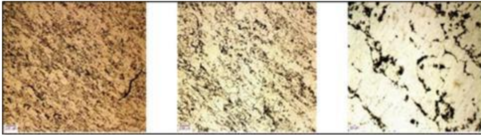
Figure 42 Microstructure of AA7055-T6 aluminium alloy at Magnification of X50, X100, X500 when impacted at 100kPa (C1)
