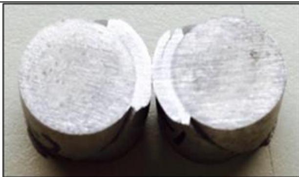
Figure 35 Crack failure of AA7055-T6 Aluminium alloy
