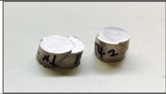
Figure 34 Failure of AA7055-T4 Aluminium alloy (side view)
