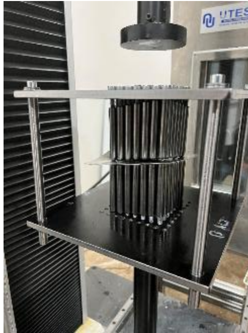
Figure 6 The die and sheet during the forming process
