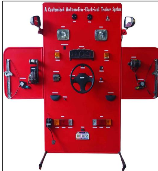
Figure 1 The Fabricated Customize Automotive Trainer System
