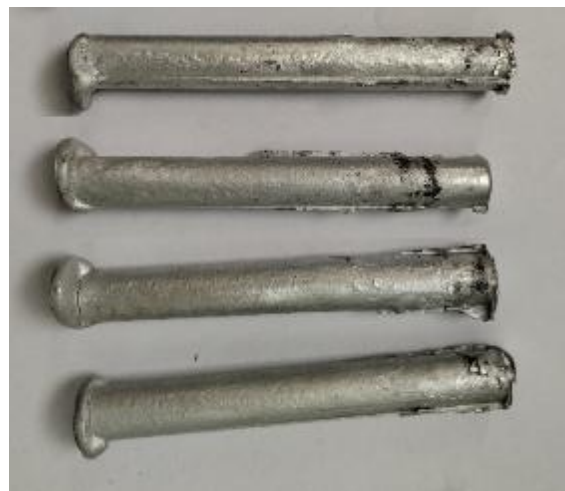
Figure 4 Al-7075 composites reinforced with B 4 C, ZrO 2 , and graphite.
