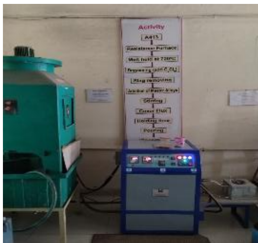
Figure 3 Stir-casting setup for Al-7075 composite fabrication.
