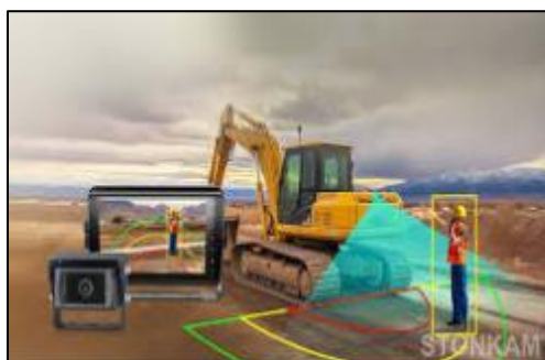
Figure 1 Rear View Camera System on Excavator
