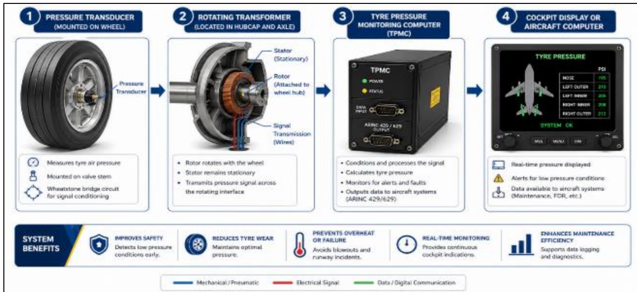
Figure 2 Aircraft Tyre Pressure Monitoring System
