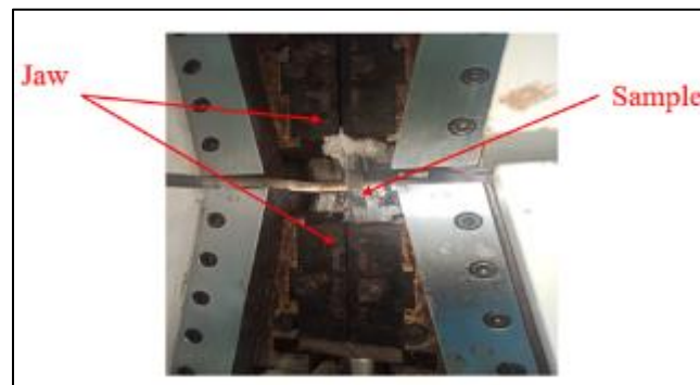
Figure 3 Tensile test setup
