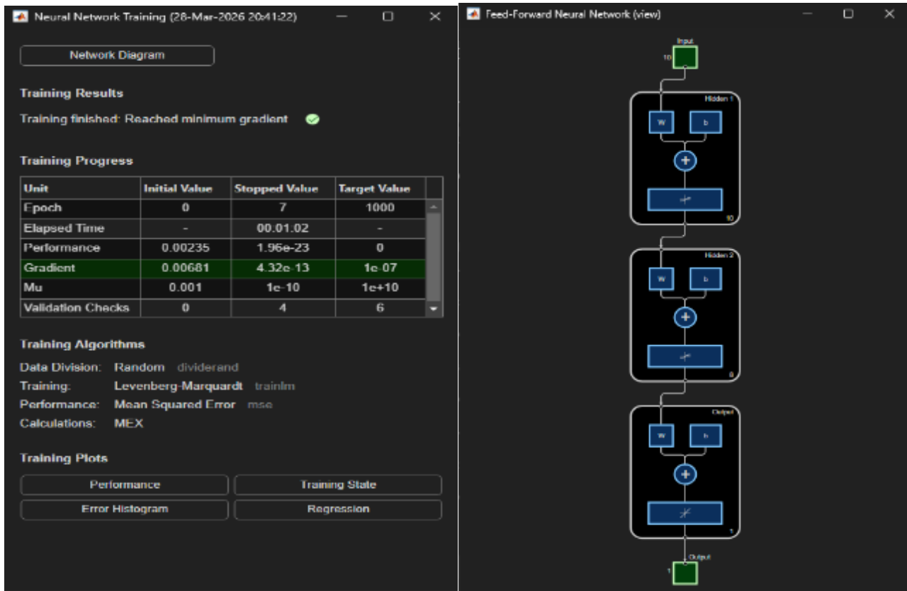
Figure 1 Neural Network Training and Structure showing input, hidden layer and output
