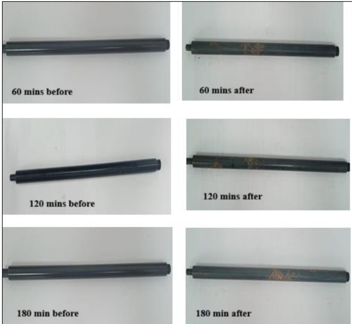
Figure 4 Red rust formation of QPQ Salt bath nitrided EN8 Steel for Nitriding Time of 60 mins,120 mins and 180 mins by salt spray test
