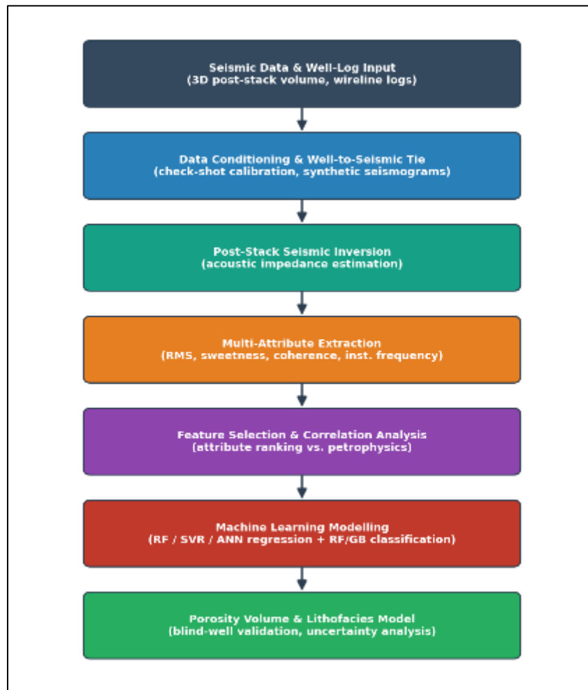
Figure 1 Integrated machine learning workflow for seismic attribute-based porosity prediction and lithofacies classification.
